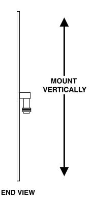
Figure 1 Antenna Mounting
