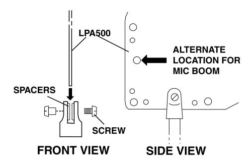
Figure 2 Microphone Stand Adapter
