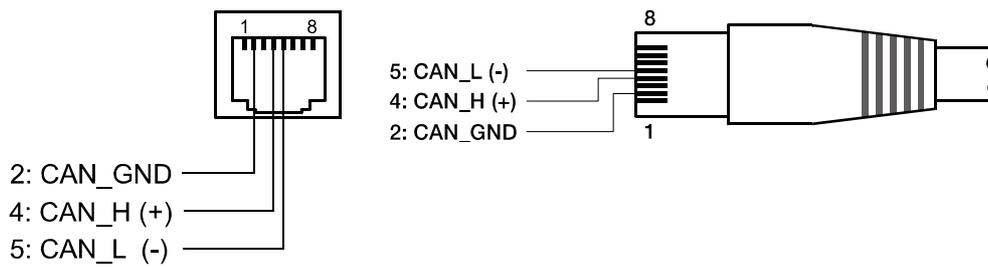
Illustration 4.2: Pin-assignment of CAN jack and CAN plug
