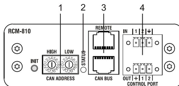
Illustration 4.1: Controls and Connections of the RCM-810
