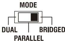
In BRIDGED mode both amp channels work in push-pull operation to provide doubled output voltage. The audio signal has to be applied to the input connectors of channel 1, amplification is set via input level control of channel 1 only.
