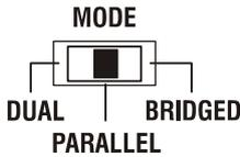
In PARALLEL mode, the inputs of channel 1 and channel 2 are directly electrically linked. The audio signal has to be applied to the input connectors of channel 1. Using the input level controls to independently control the amplification of the two channels is still possible because only the channels' inputs are linked. PARALLEL operation is the mode of choice, whenever the same input signal drives multiple power amp channels of a large system installation.
