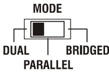
In DUAL mode, the two channels of the power amplifier work independent from each other. This mode of operation is being used for all 2-channel applications, like stereo operation. Using the input level controls on the power amp's rear panel allows independently adjusting the channels' amplification.
