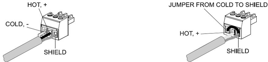
Illustration 2.1: Balanced / unbalanced connection of input
