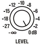
In DUAL and PARALLEL mode, the level controls LEVEL on the power amp's rear panel are used to control the amplification of the corresponding channel. Turning the control to the right increases and turning it to the left decreases the volume. In BRIDGED mode operation, the output volume of the power amp is only controlled by the CH 1 level control. Any changes in the setting of the CH 2 level control are ignored.
