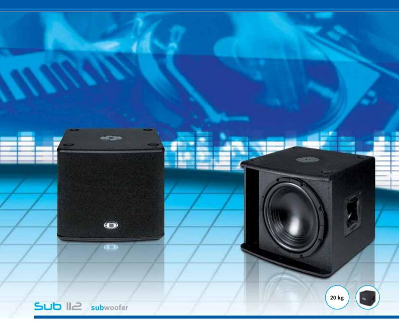
The DYNACORD SUB 112 is a vented, direct-radiating cabinet equipped with a high-power DYNACORD DND12S400 neodymium woofer boasting power handling of 400W (rated) and 1600W (peak). The conical vent system results in less flow loss and lower air noise than conventional vented designs. High sound pressure levels are also generated at low frequencies with significantly less distortion than by conventional bass reflex vents.
