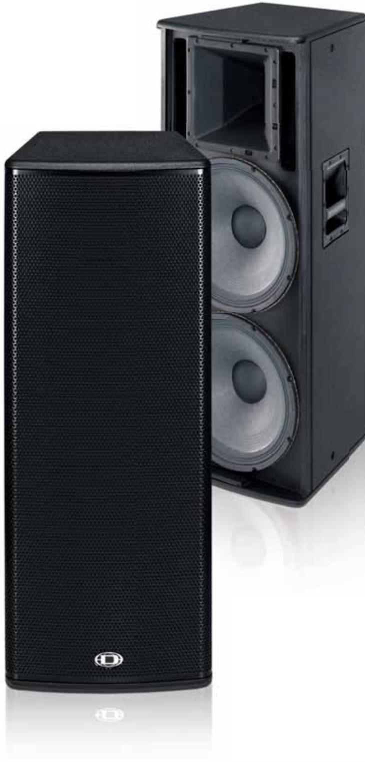
■ If very high sound pressure levels are required from a compact format, the trapezoidal C 25.2 double 15" / two-way full-range cabinet is the ideal choice, with its very high power handling (1000W continuous / 4000W peak) and sensitivity of 103 dB 1W / 1m.
