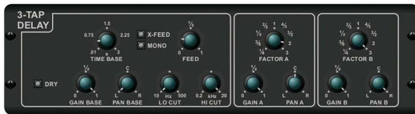
The 3-TAP DELAY in the M32 records the input signal and then echoes it back after a user-definable period of time and number of repeats. What makes the stereo and triple delay useful and outstanding is the linked tap-timing and musical choice of echo patterns.
