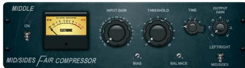
The Fairchild 670 tube compressor not only achieves record bids in high-end vintage gear auctions, it also delivers some of the finest colorations in compressor history. Two small trim VR's preset the control side chain action, a six-step switch determines the timing, and the two large Input and Threshold knobs adjust the levels.
